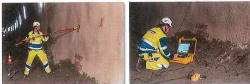
Figure 3 Simple installation of receiver and recording unit of the TSP 303 system.
