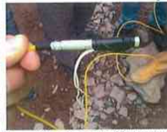
Figure 4 Detonator cap with wrapped round wire (white) that gives the accurate recording trigger in the moment of blast.
