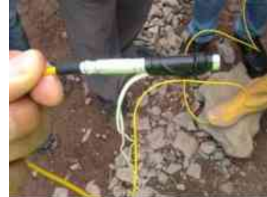
Figure 5 Detonator cap with wrapped round wire (white) that gives the accurate recording trigger in the moment of blast.
