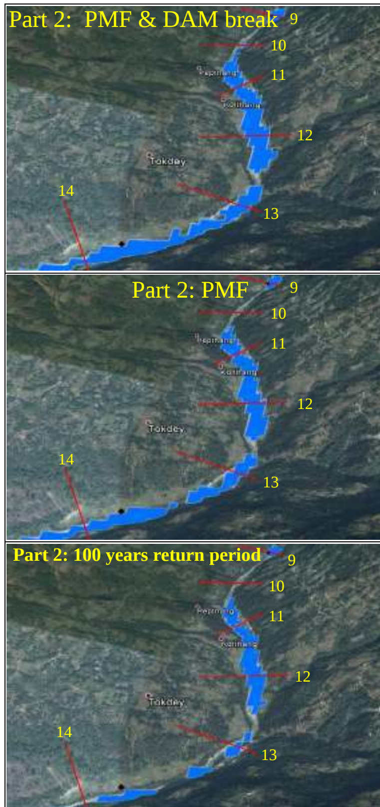
Figure 6.10: Flood inundation at Part 2
