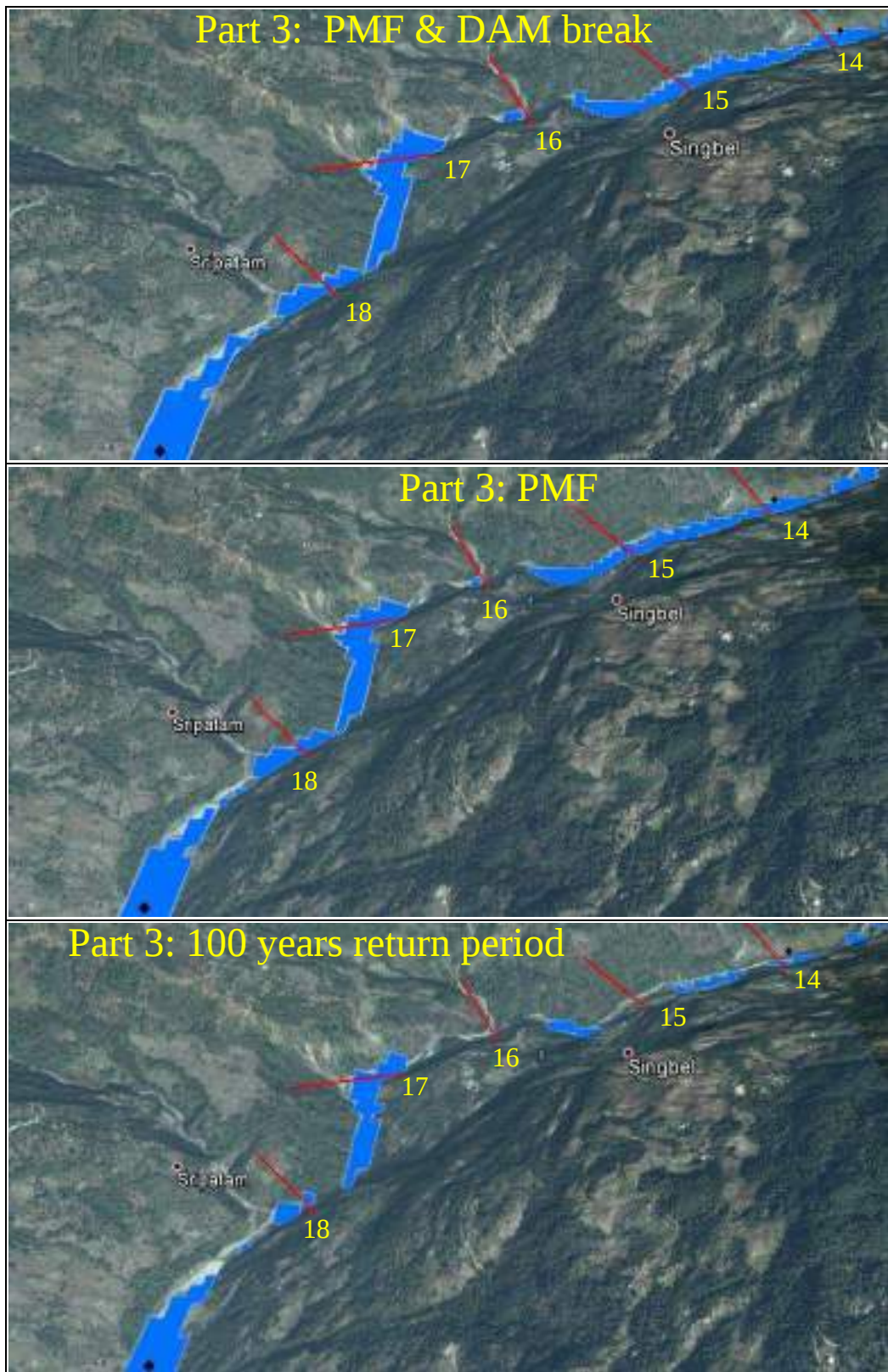
Figure 6.11: Flood inundation at Part 3
