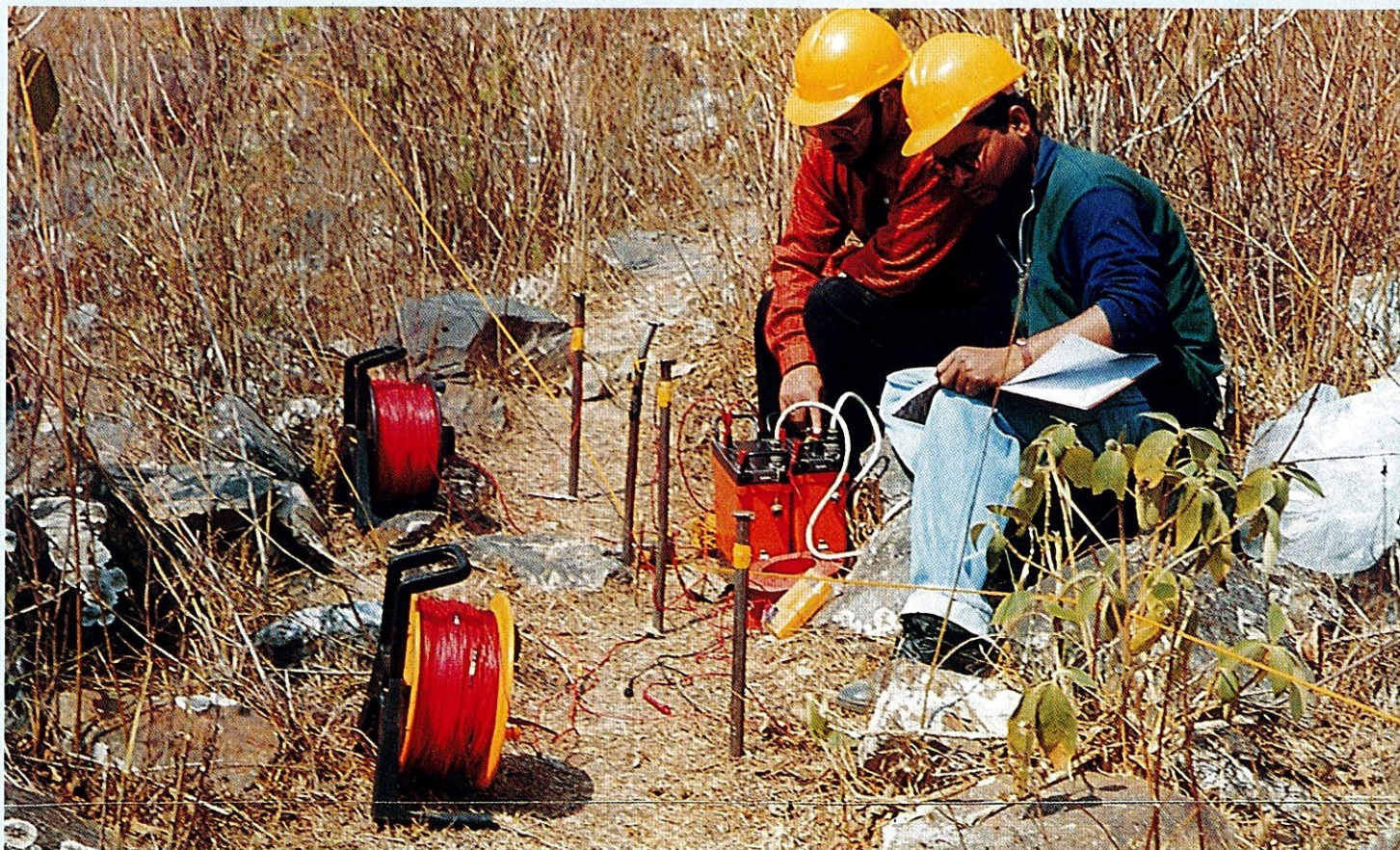
Resistivity measurement for ground water studies and earthmat design utilising SAS Terrameter.
